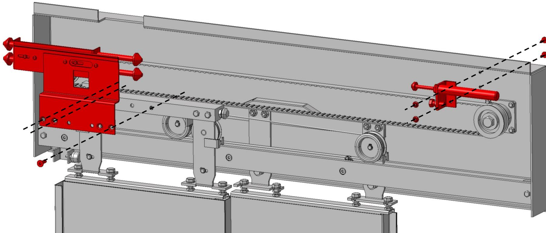
Demontage: Bauteile die entfallen (rot dargestellt) / Disassembly: Components being omitted (shown in red)
