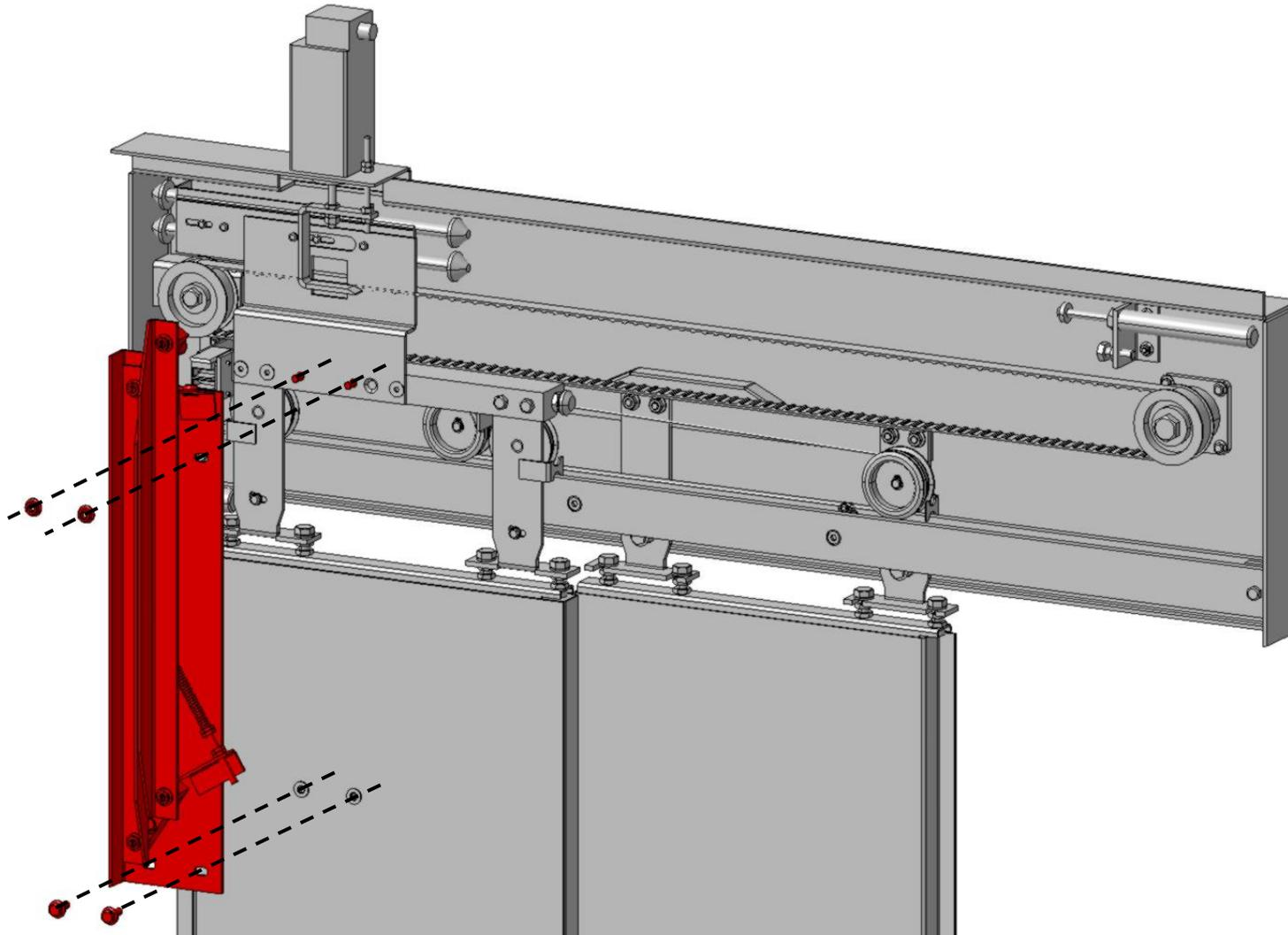
Demontage: Bauteile die entfallen (rot dargestellt) / Disassembly: Components being omitted (shown in red)
