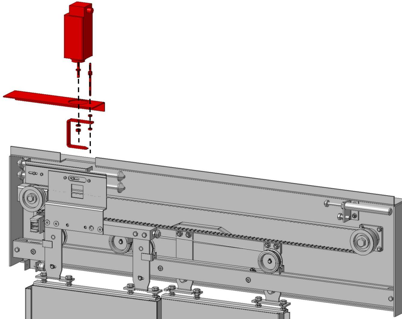
Demontage: Bauteile die entfallen (rot dargestellt) / Disassembly: Components being omitted (shown in red)
