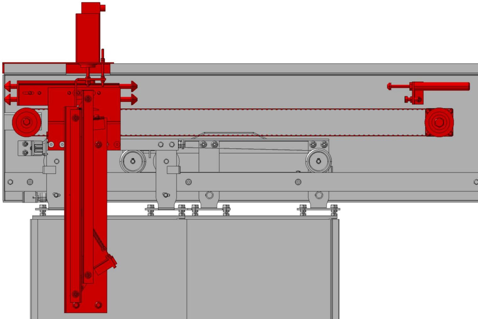
Demontage: Bauteile die entfallen (rot dargestellt) / Disassembly: Components being omitted (shown in red)
